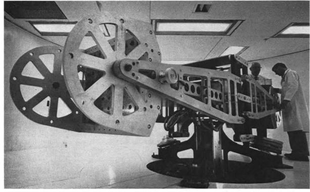
CENTRIFUGE sunken in the floor of Bldg. 860 is used for sustained acceleration tests of components. H. G. Page (left) and D. J. Adkins mount a test unit at far end which will be balanced by weights or another unit on the foreground arm of the centrifuge. The machine is capable of developing 150 g's of acceleration on test units weighing up to 200 lbs. Rate is 270 revolutions per minute.
